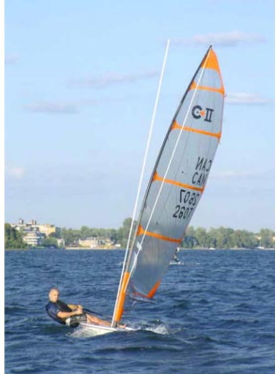
The most flexible of the masts showed excessive side bend in the lower third.
