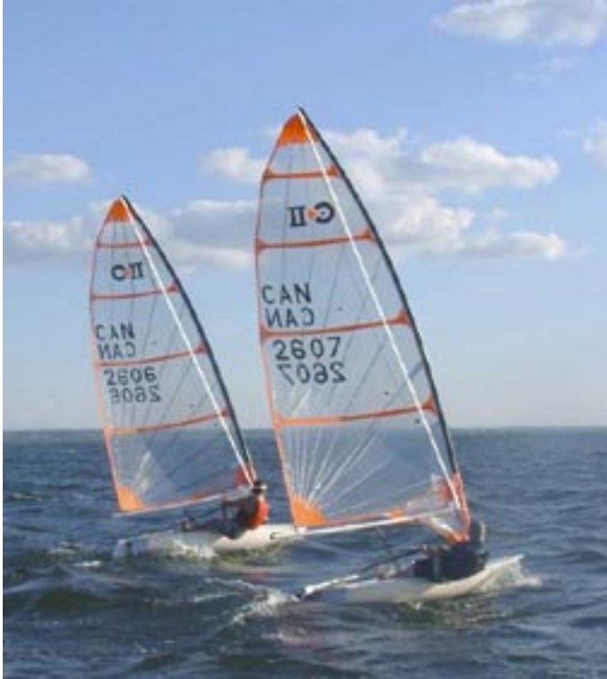
Marc-André Littée and brother Pat do boat for boat testing in 16-18 kts. Pat to weather has one of the Australian flexible masts and Marc-André has the UK mast. Notice that the boat is not as flat - both brothers are identical weight. White lines are overlaid on the photographs and were scaled after testing to accurately assess mast bend.
